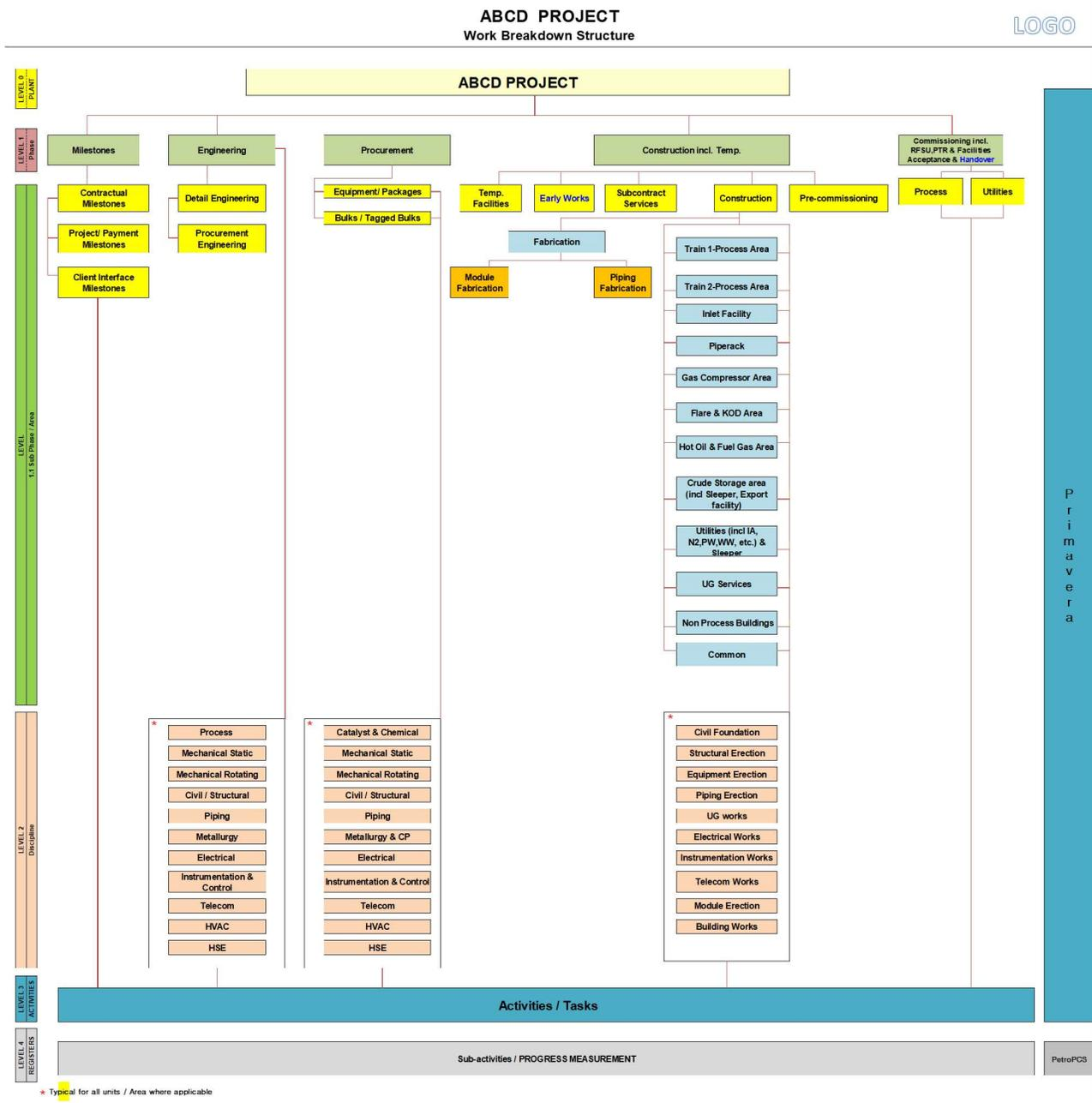
Figure4: Typical Work Breakdown Structure
