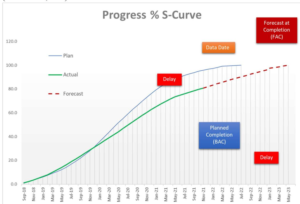
Figure-1: Progress S-Curve reflecting the actual progress behind the plan
