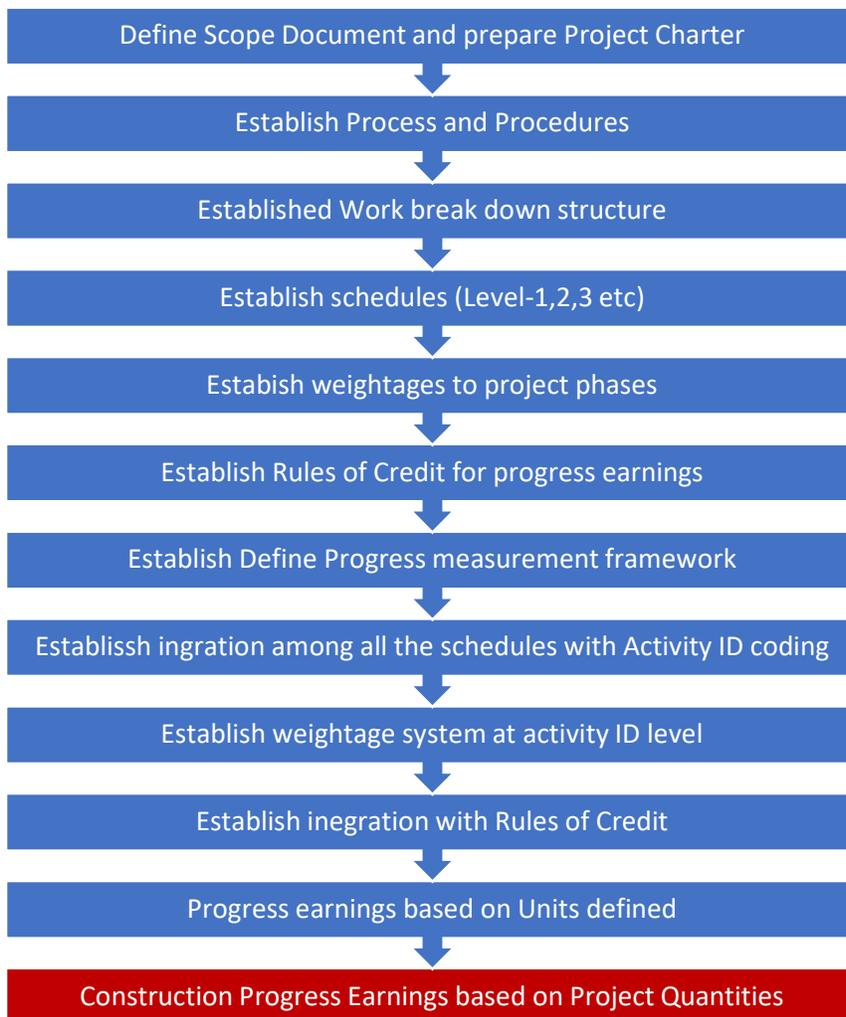
Figure-3: Project Progress Measurement Process Hierarchy
